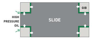
Slide remains centered F-B & R-L with Hydrostatic/Hydrodynamic guiding
