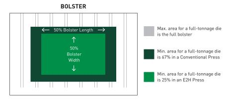
Minimum area for a full-tonnage die in a Minster E2H is almost 50% less than a typical press
